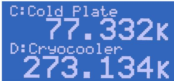
Several display formats may be selected. Up to eight temperature readings may be displayed simultaneously or two channels with input names and temperature shown in a large easy to read font. Additional screens include temperature readings along with relay and alarm status information.
